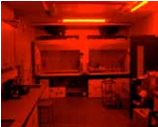
Much of the year is based in the Oxford Luminescence dating laboratory (left) where sediment must be prepared in red light conditions to prevent the depletion of a luminescence signal prior to measurement (right).
